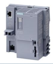
SIMATIC DP, CPU 1512SP F-1 PN for ET 200SP, central processing unit with 600 KB work memory for program and 2 MB for data, 1st interface: PROFINET IRT with 3-port switch, 6 ns bit performance, SIMATIC Memory Card required, BusAdapter required for port 1 and 2
