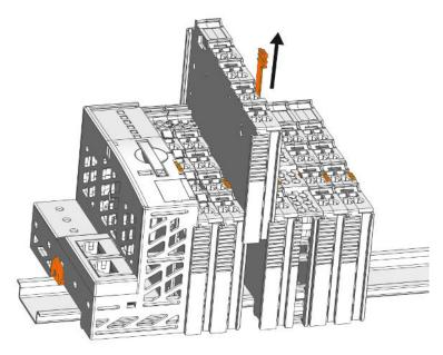
Figure 28: Pulling the Release Tab
