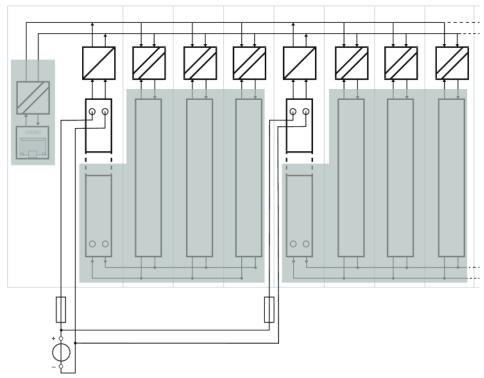
Figure 13: Supplying System Power (Example)
