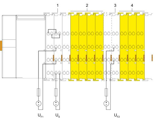
Figure 22: Power Supply Concept Example with F I/O-Modules
