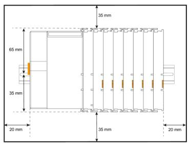
Figure 15: Installation Clearances
