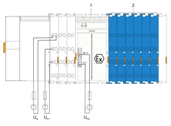
Figure 19: Ex i Power Supply Concept
