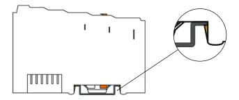
Figure 11: DIN-Rail Contact (example)
