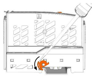
Figure 23: Locking the Head Station
