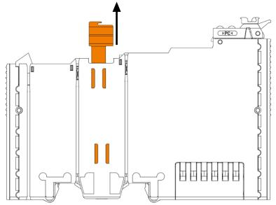
Figure 30: Detaching the 753 Series I/O Module
