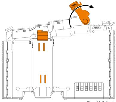
Figure 29: Pulling the Locking Latch
