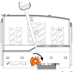
Figure 27: Disengage the locking cam
