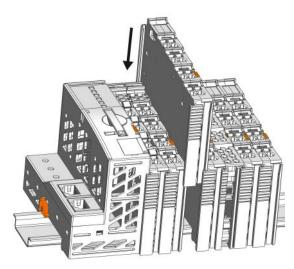
Figure 25: Snapping the I/O Module On
