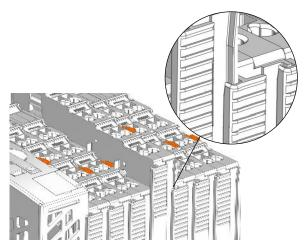
Figure 24: Inserting the I/O Module
