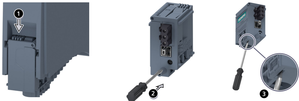
Figure 8-6 Connecting the supply voltage to a system power supply/load current supply (1)
