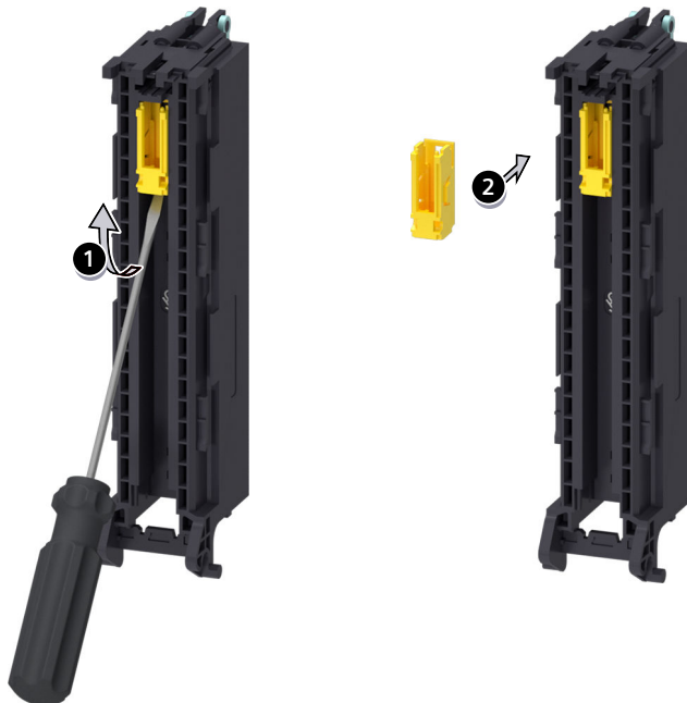
Figure 15-10 Removing the electronic coding element from the front connector and inserting it into a new front connector
