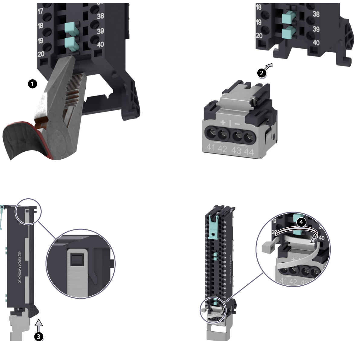
Figure 8-12 Preparing front connectors for I/O modules with shield contact element (1)
