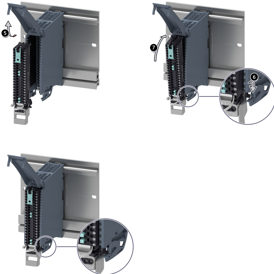
Figure 8-13 Preparing front connectors for I/O modules with shield contact element (2)
